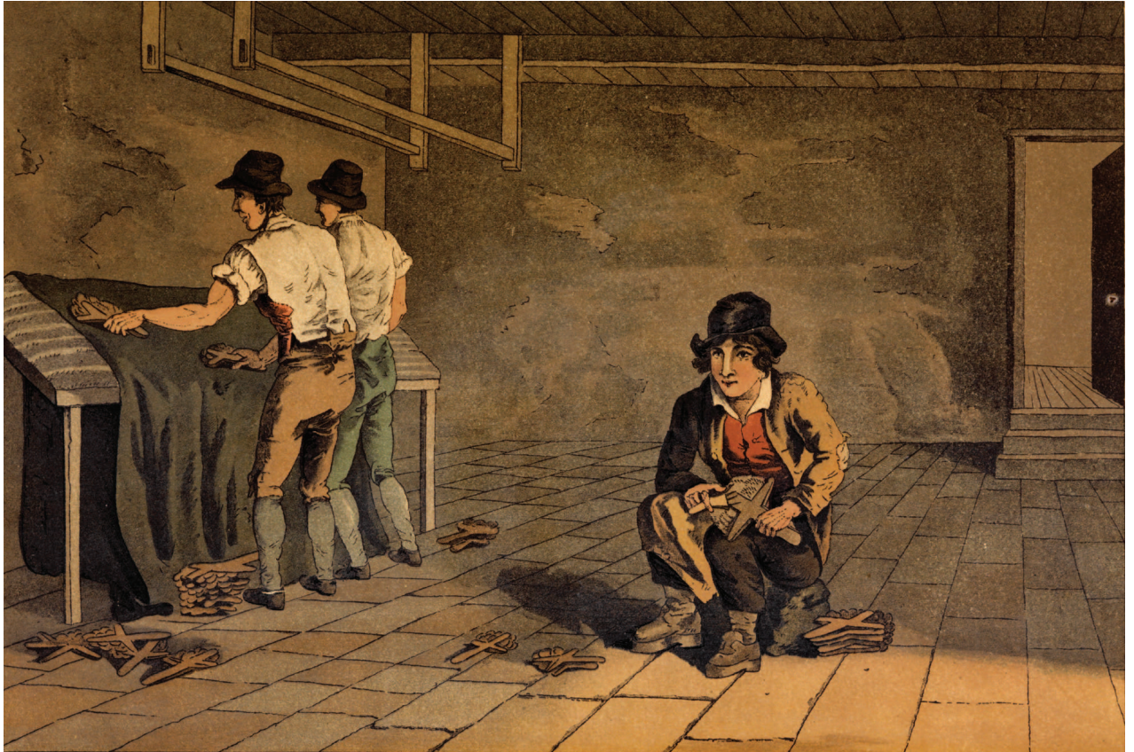
This scene from George Walker's The Costume of Yorkshire , 1814, here taken from Edward Hailstone's edition of 1885, shows croppers at work in a Leeds dressing shop raising broadcloth with teasles. After both sides of the handles had been used, they were cleaned of flock by a small boy with a spiked tool called a preem. (Reproduced by kind permission of the Dean and Chapter of York)
